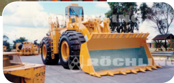
Bucket liners made of Matrox®
