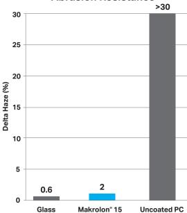
\*Taber Abrasion per ASTM D 1044, 100 cycles, CS-10F wheel
