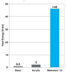
\*Instrumented Impact per ASTM D 3763, sample thickness 0.125 " nominal
