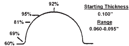
Wall Thickness of Sheet Formed in Cylindrical Male Mold
